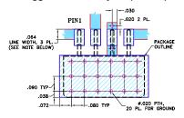
NOTES: 1.TRACE WIDTH IS SHOWN FOR ROGERS R04350B WITH DIELECTRIC THICKNESS 0.030" ± 0.002"; COPPER: 1/2 0.2 EACH SIDE. FOR OTHER MATERIALS TRACE WIDTH MAY NEED TO BE MODIFIED.
